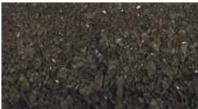
The sample crushed in a jaw crusher has a particle size of approximately 8 mm..
